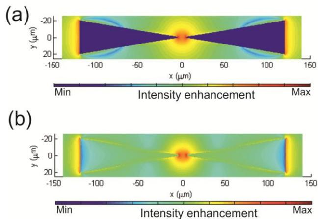
**Fig 1:** Simulated near-field intensities for axial THz illumination on bow-tie antennas showing enhancement of near-fields in (a) gold and (b) doped-Si both on quartz substrate. The intensity is calculated at the upper surface of the antennas.
